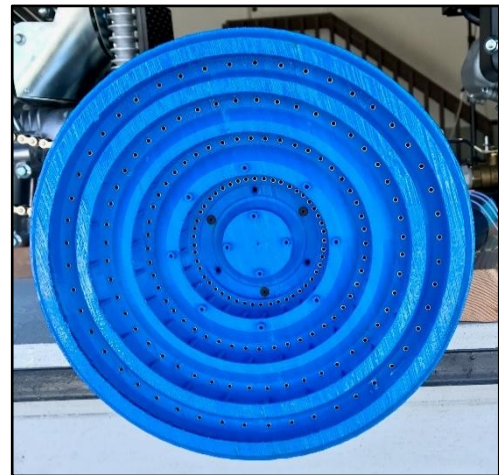
Figure 6. DiscThruster plan view shows four circumferential rows of rocket nozzles.
