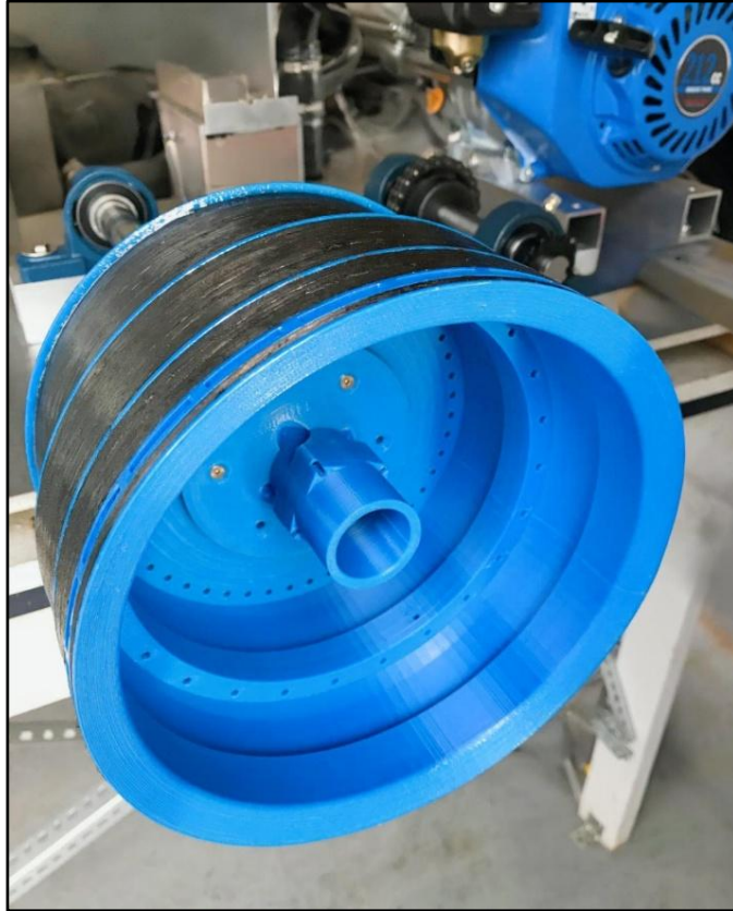
Figure 10. DiscThruster's closed cycle design exhibits two sets of nozzle rings and a composite structural overwrap.
